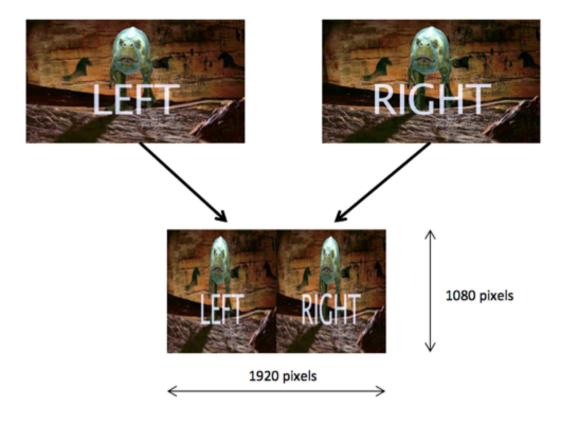
The two genuine HD pictures (left and right eyes) are squeezed horizontally by anamorphosis to have a format 960x1080, then both are juxtaposed (left eye on the left side, right eye on the right side) to make a new complete picture which format is 1920x1080.
